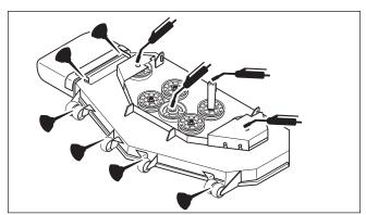
Figure 18. Deck Lubrication
